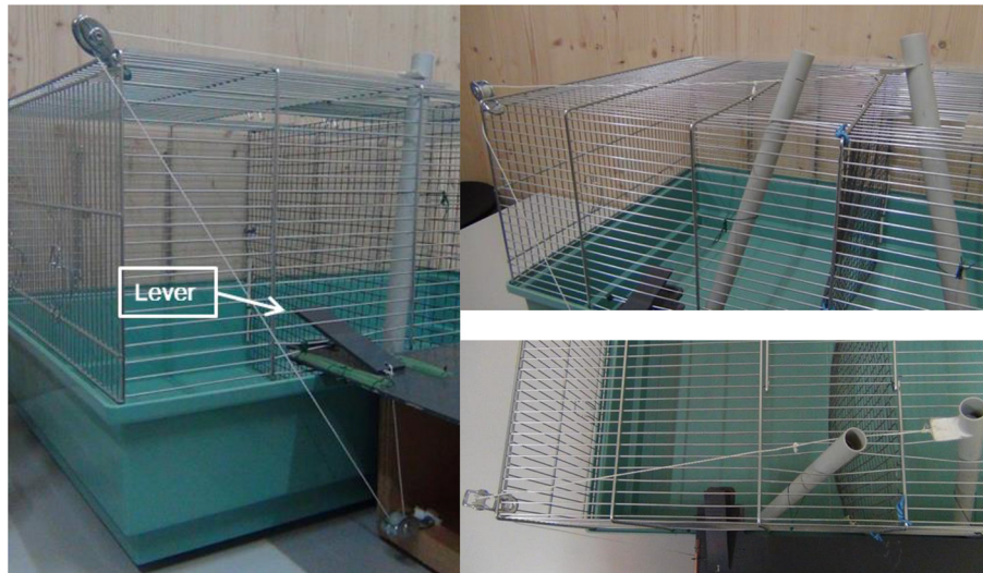
Figure A1. Pushing mechanism. When the rat pushed the lever, a trapdoor in the grey plastic tube opened releasing a food item which fell into the partner's compartment.
